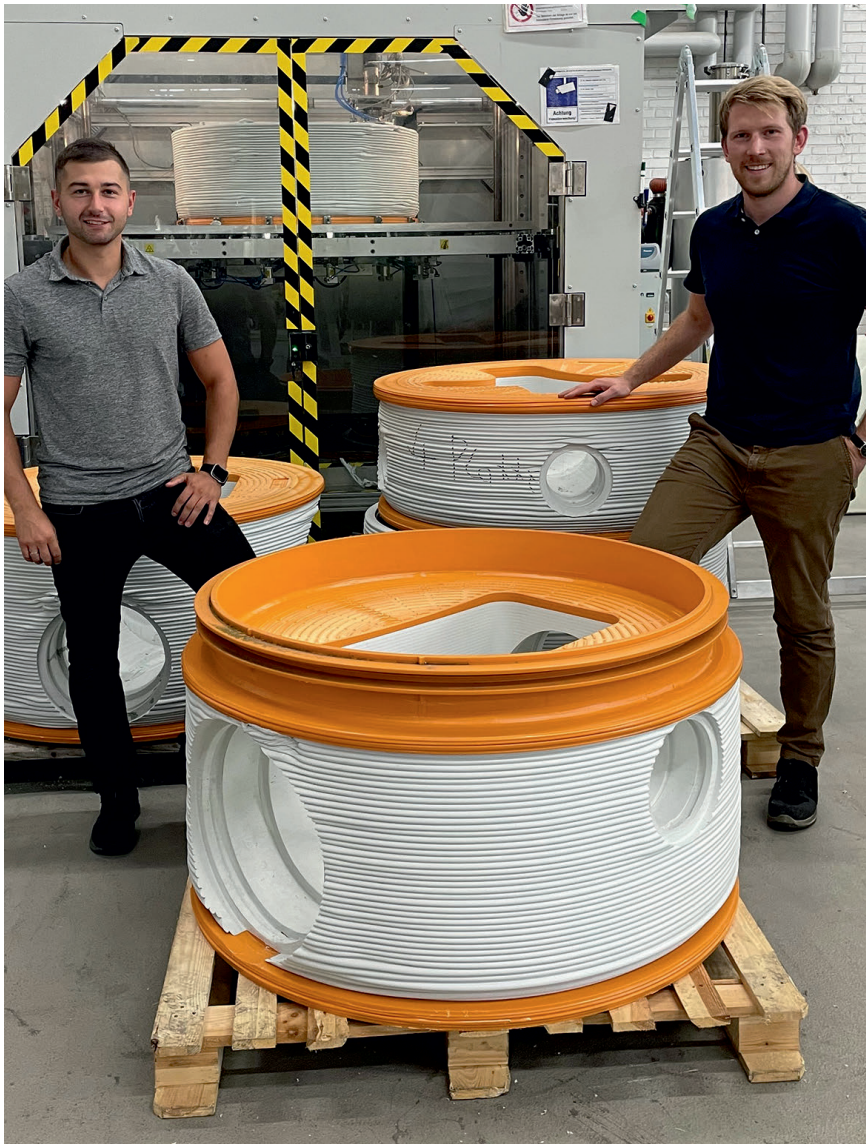
Kevin Winter (left) and Jonas Wilfert from Rehau in their 3D printing production environment. Components can have a maximum diameter of 1.2 m and height of 85 cm © Rehau
